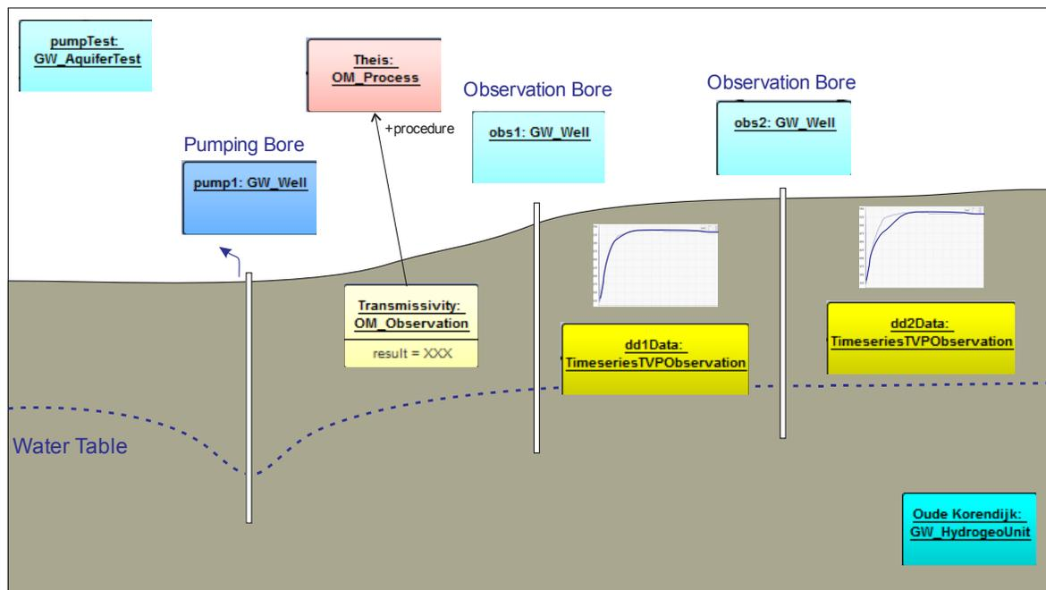
Figure 22: Typical setup of a pumping test.
