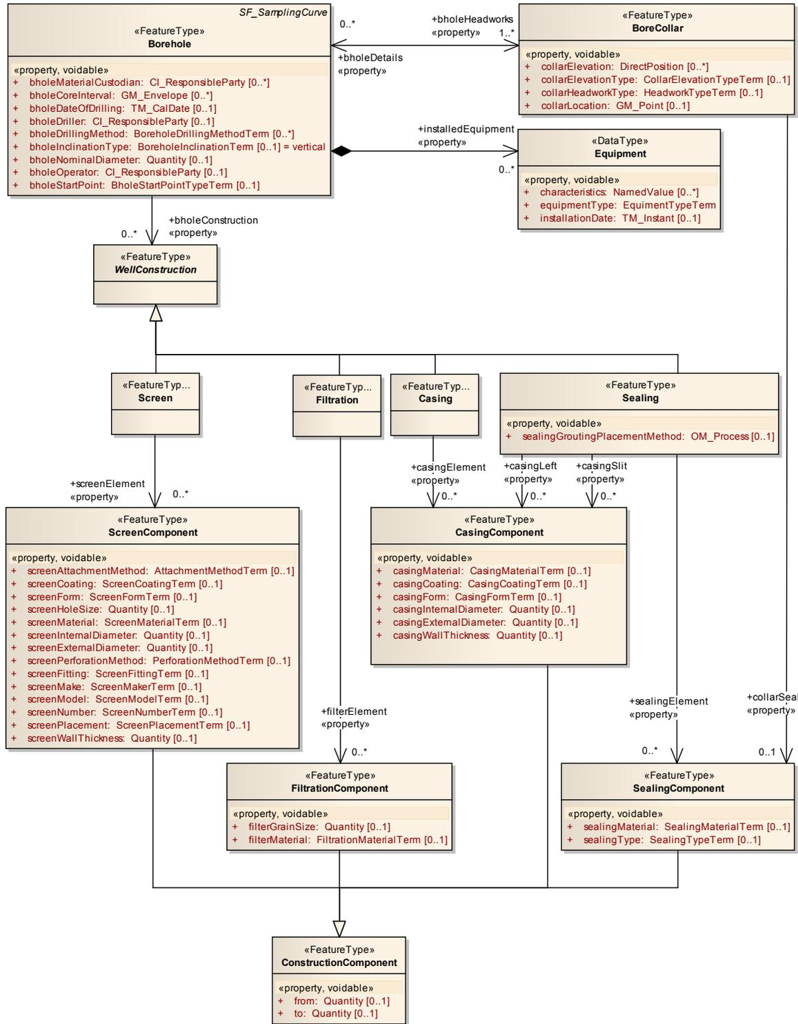
Figure 15: GWML2 LM - WellConstruction.
