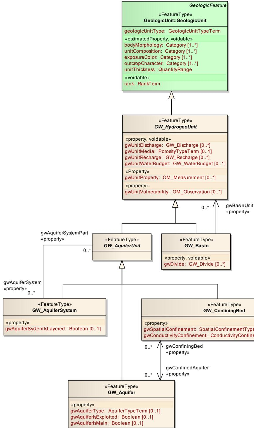
Figure 9: GWML2 LM - Hydrogeological Unit.
