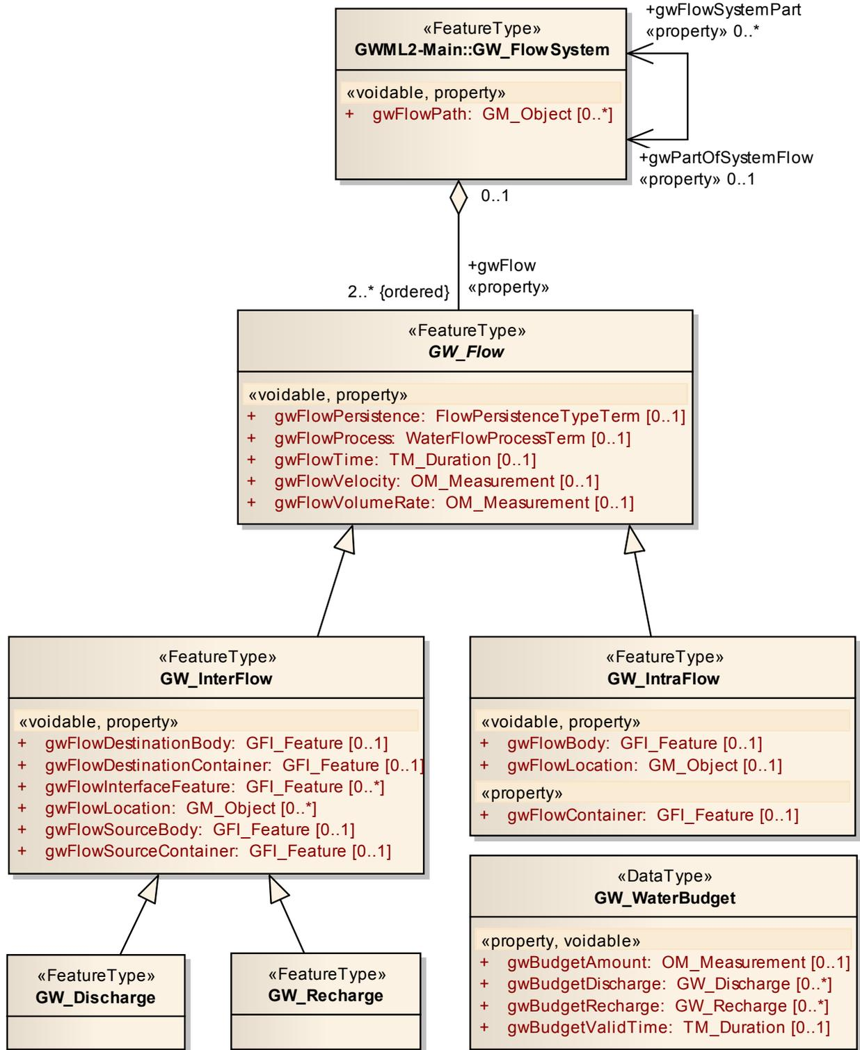
Figure 13: GWML2 LM - Groundwater Flow.
