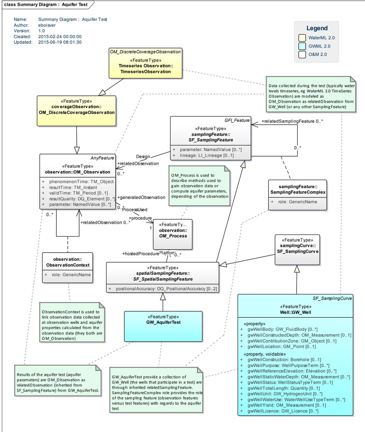
**Figure 21: Summary diagram for aquifer tests, a profile of Observations and Measurements.**
