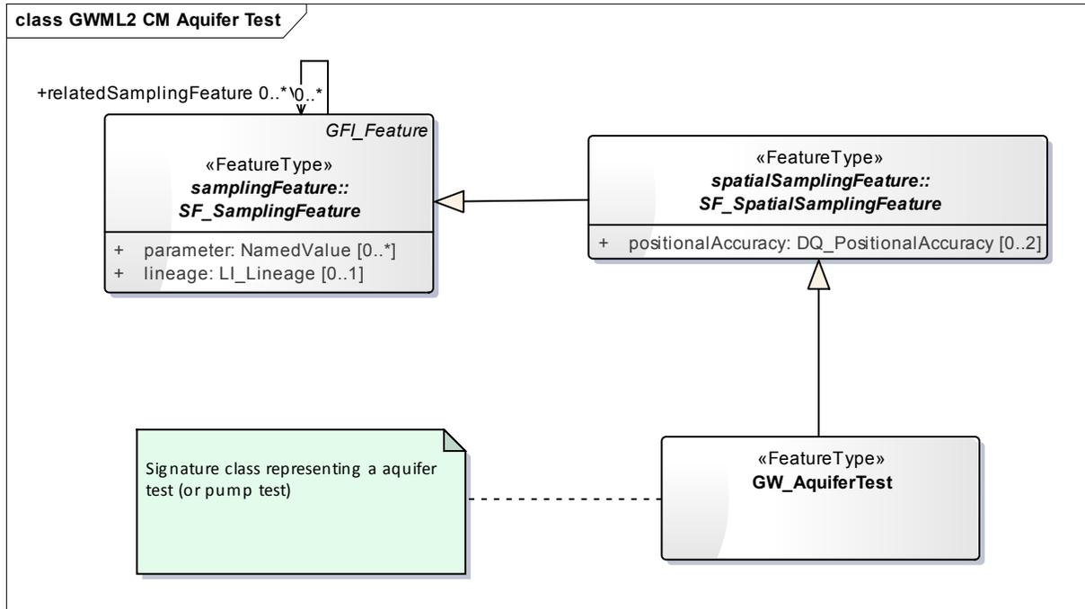
Figure 23: GW\_AquiferTest model.
