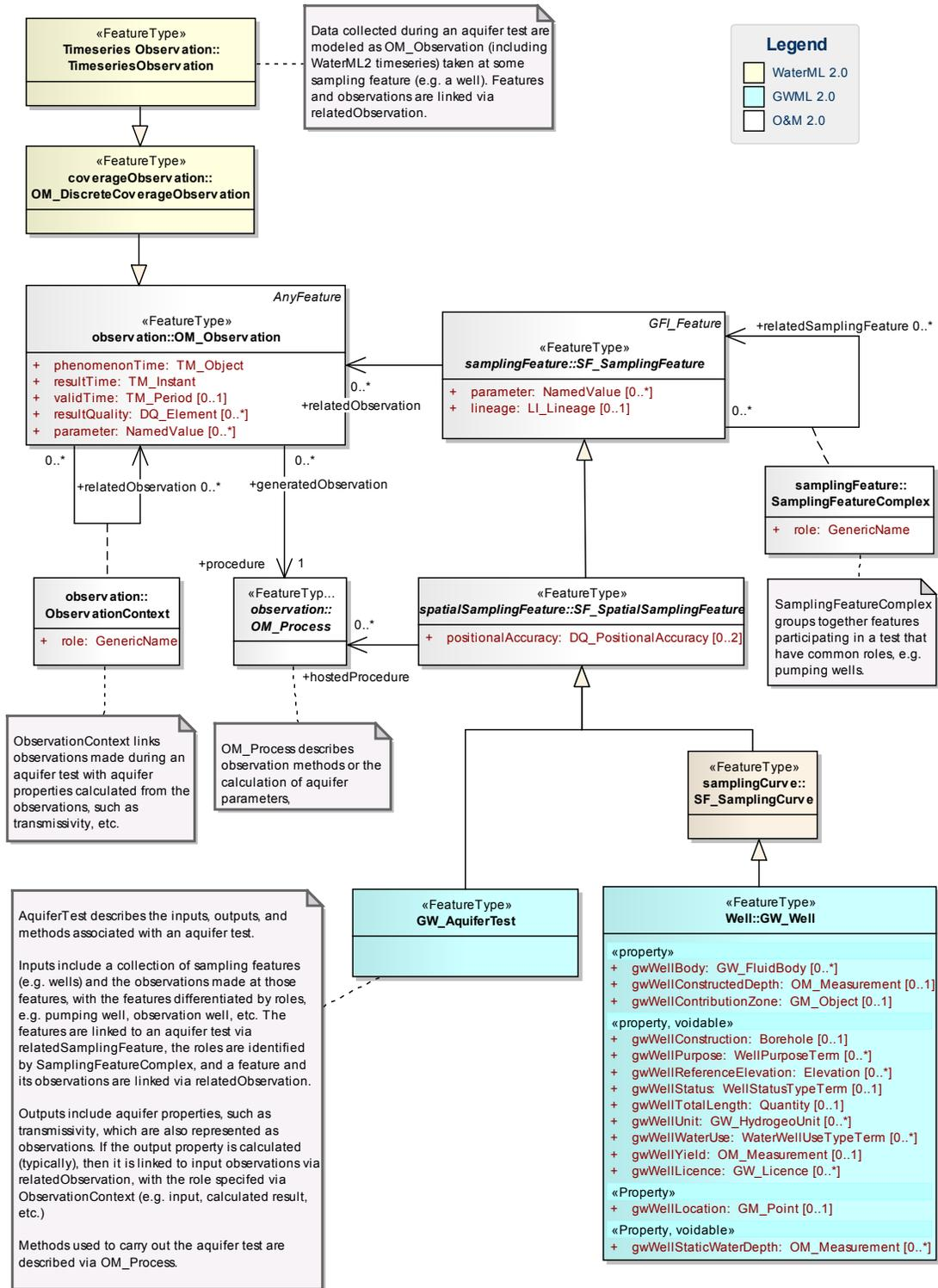
Figure 16: GWML2 LM - Aquifer Test.
