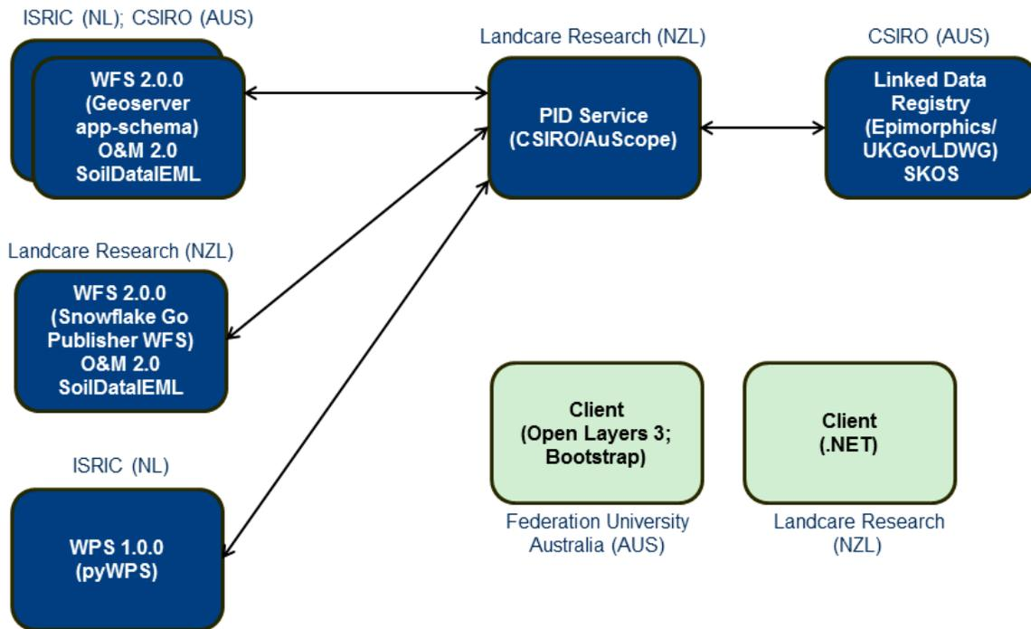
**Figure 14 — Overview of Demonstration 1 components.**
